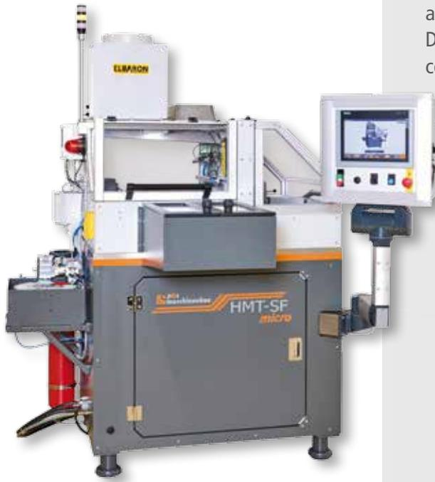
The HMT-SF micro is a fully automated system which was developed for cutting and chamfering smallest round bars made of a wide variety of materials such as carbide, hss, ceramics, etc..
