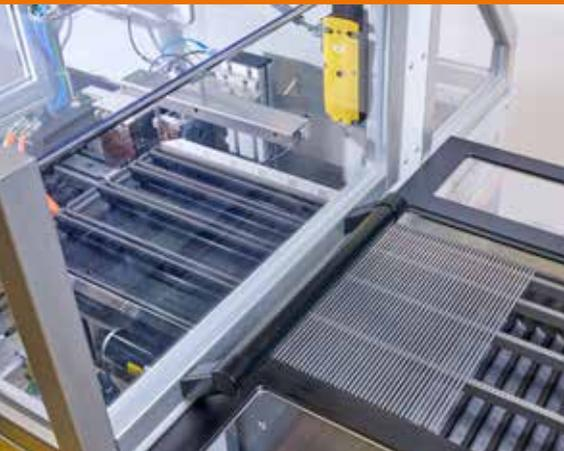
Blanks are getting placed in the outside magazine either manually by hand or automated
