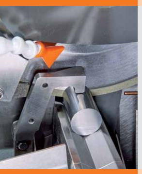
The HMT-S15 is the standard machine in our product line for separating carbide and HSS. The production area lies between  $\emptyset$  3 mm -  $\emptyset$  40 mm. With a large and easy-to-load magazine, it is ideal for medium to large quantities. The best tried-and-tested P&S separation technology is installed.
